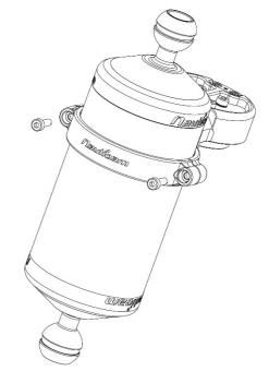
2. Place a float arm and the bracket as shown, then secure the bayonet holder by tightening the two screws.
