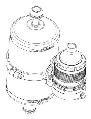
3. Align the 'I' mark on the bayonet holder with 'O' mark on the EMWL Objective lens and then push it in.
