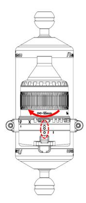
4. Turn the EMWL objective lens clockwise until 'O' mark on the lens aligns with the 'O' dot on the bayonet holder and a 'click' sound is heard.
