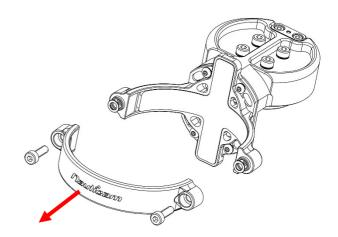
1. Remove the bracket from the bayonet holder by unscrewing the two screws.
